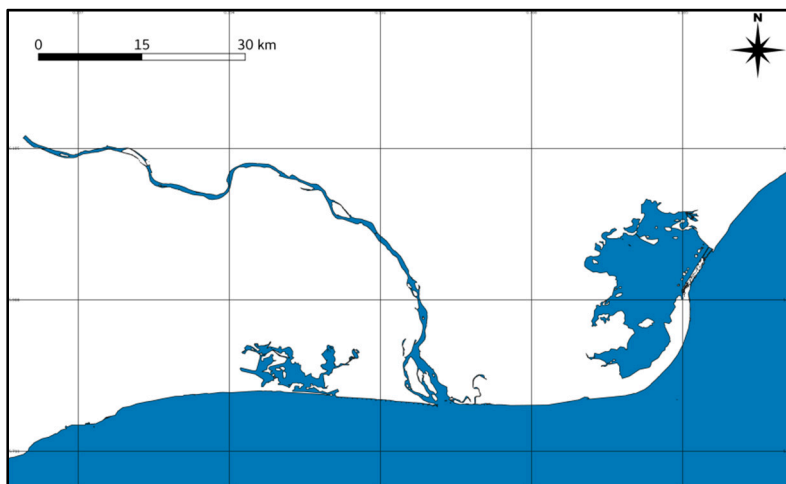
Figure 4. A section of a Ghana land–water mask generated using Sentinel-1 SAR data (from left to right: Songaw Lagoon, River Volta, and Keta Lagoon).
